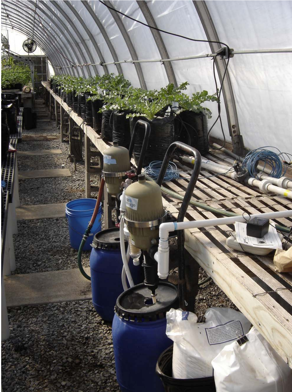
Figure A-21: Hydroponic apparatus in greenhouse used to determine the effects of water stress on milk thistle ( Silybum marianum ) plants.
